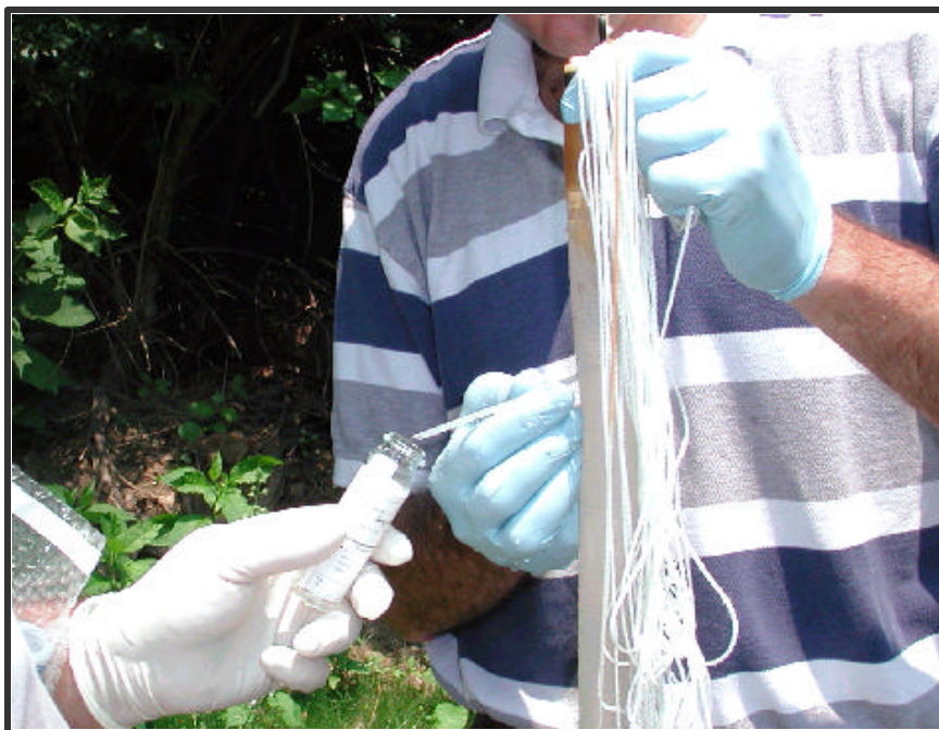
Figure 2. Zero-Purge Sample Collection
