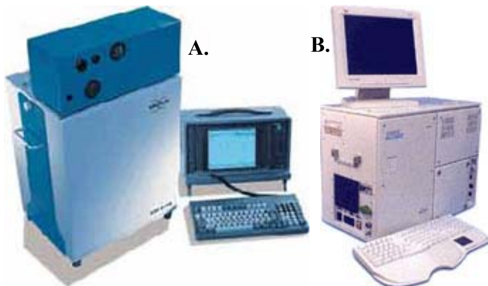
Figure 6. Transportable GC/MS instruments (A) EM640™ Mobile GC/MS; (B) The Viking 573 GC/MS. ( http://www.bdal.de/modux3/ ). Photos used with permission.
