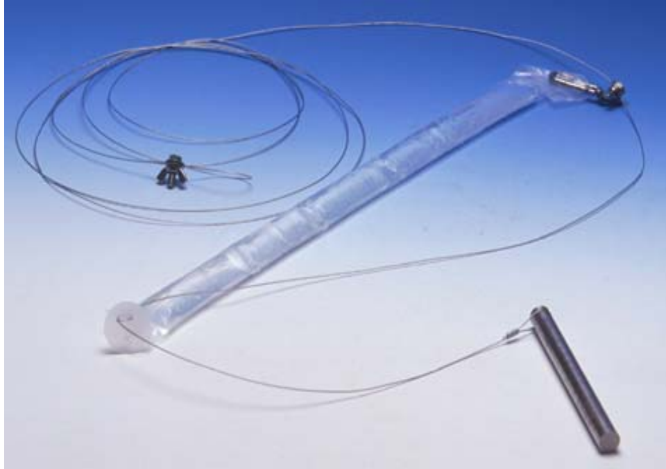
Figure 1. The passive diffusion bag sampler. Photo used with permission. ( http://www.caslab.com/products.php )
