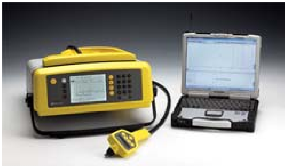
Figure 5. The HAPSITE ® Quadrupole GC/MS. Photo used with permission. ( http://www.inficonchemicalidentificationsystems.com/hapsitechemicalidentification.html )
