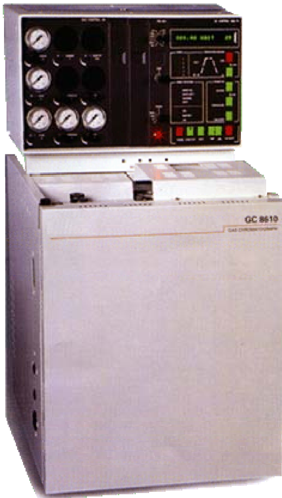
Figure 4. Model 8610 GC. Photo used with permission. ( http://www.spectrolab.co.uk/gas_chromatography/gc8160.htm )
