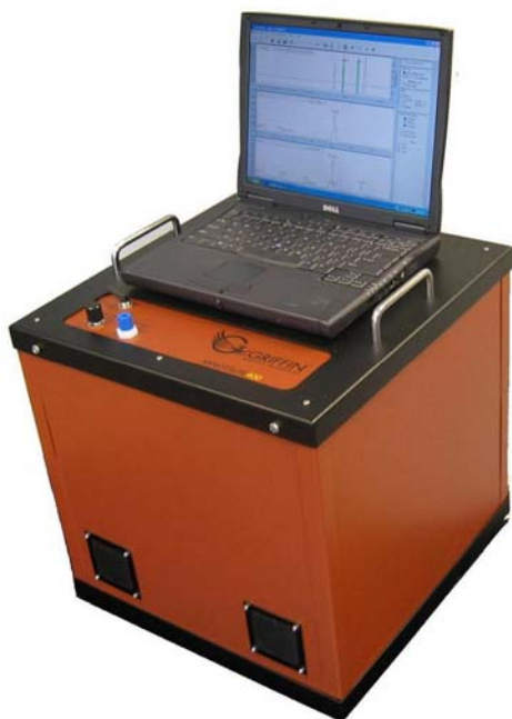
Figure 8. Minotaur 400 cylindrical ion trap mass spectrometer. Photo used with permission. ( http://www.griffinanalytical.com/main_products.html )
