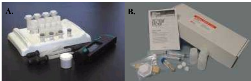
Figure 3. (A) RaPID TPH/BTEX assay kit; (B) D Tech TNT field kit. Photos used with permission.
