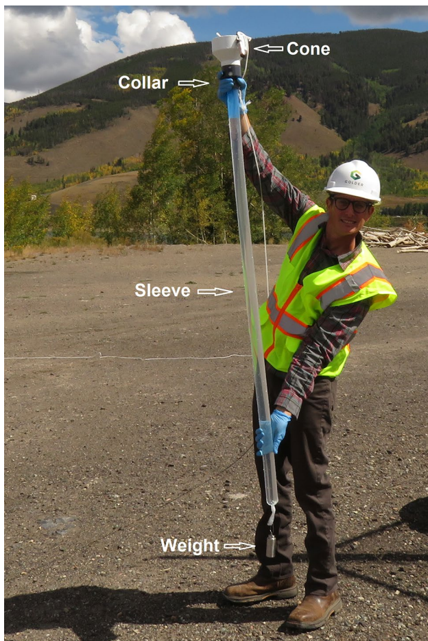
Fig. 2 A full, 1.5-m-long HydraSleeve after drone sampling
