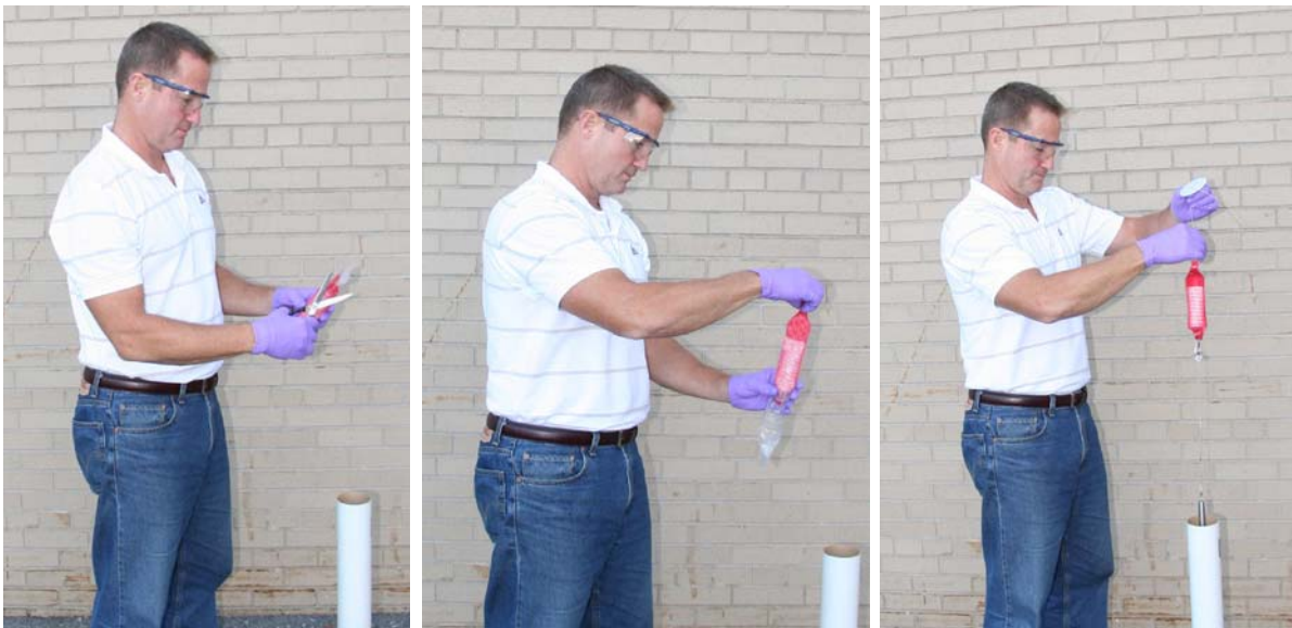
Figure 6-4. RPP sampler deployment at the wellhead.
