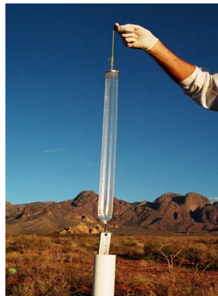
Figure 3-1. Full HydraSleeve retrieved from a well.
