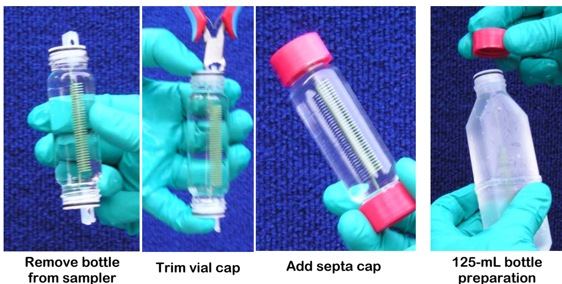
Figure 4-8. Preparation of Snap Sampler bottles. (Three photos on left show a 40-mL VOA vial. Photo on right is a 125-mL plastic bottle).
