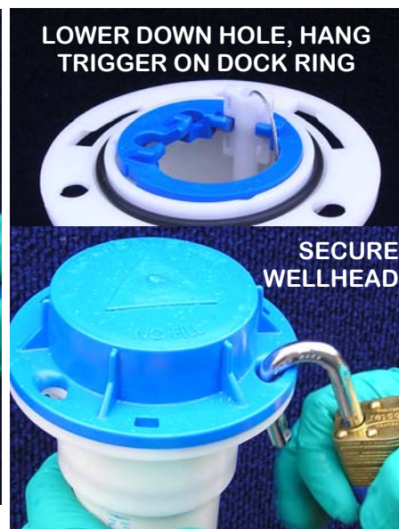
Figure 4-7. Securing sampler into wellhead docking station.
