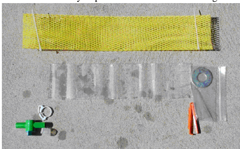
Figure 5-2. Parts of a dialysis sampler before assembly. (~2.5 inches in diameter by 24 inches long)
