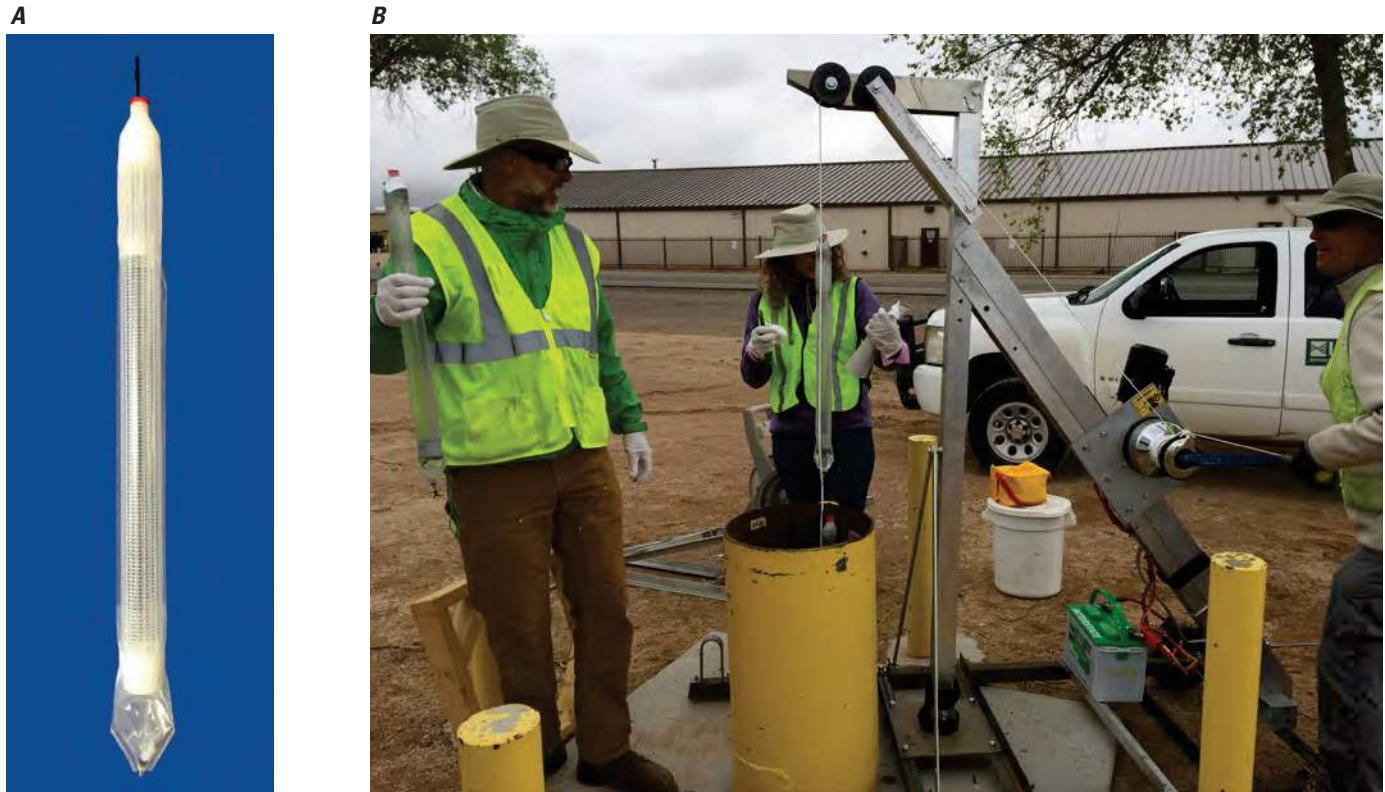
Figure 11. A, An EON Products, Inc. Dual Membrane (DM) sampler® and B, a vertical string of DM samplers being retrieved from a well. Photographs by Bradley P. Varhol, EON Products, Inc. and Rebecca Travis, U.S. Geological Survey.
