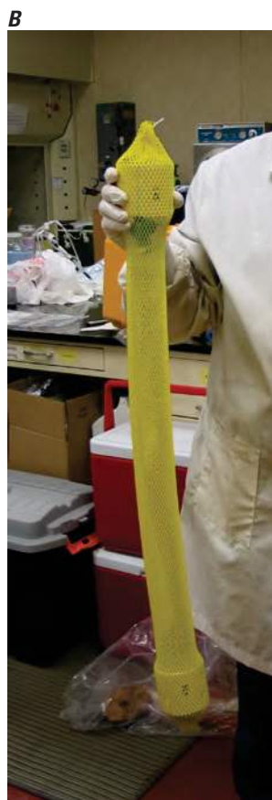
Figure 7. A 2.5-inch diameter regenerated cellulose dialysis membrane sampler with external supports, A , prior to assembly, and B , after assembly. Photographs by Thomas E. Imbriotta, U.S. Geological Survey.
