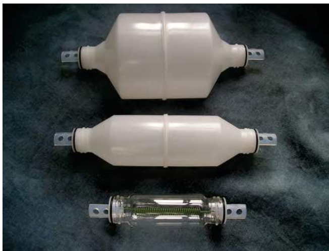
Figure 13. The QED Environmental Systems, Inc. Snap Sampler® with A, a volatile organic compound bottle (40-millileter vial), and B, variously sized volatile organic compound and inorganic constituent bottles. Photographs by Sanford Britt, QED Environmental Systems, Inc.
