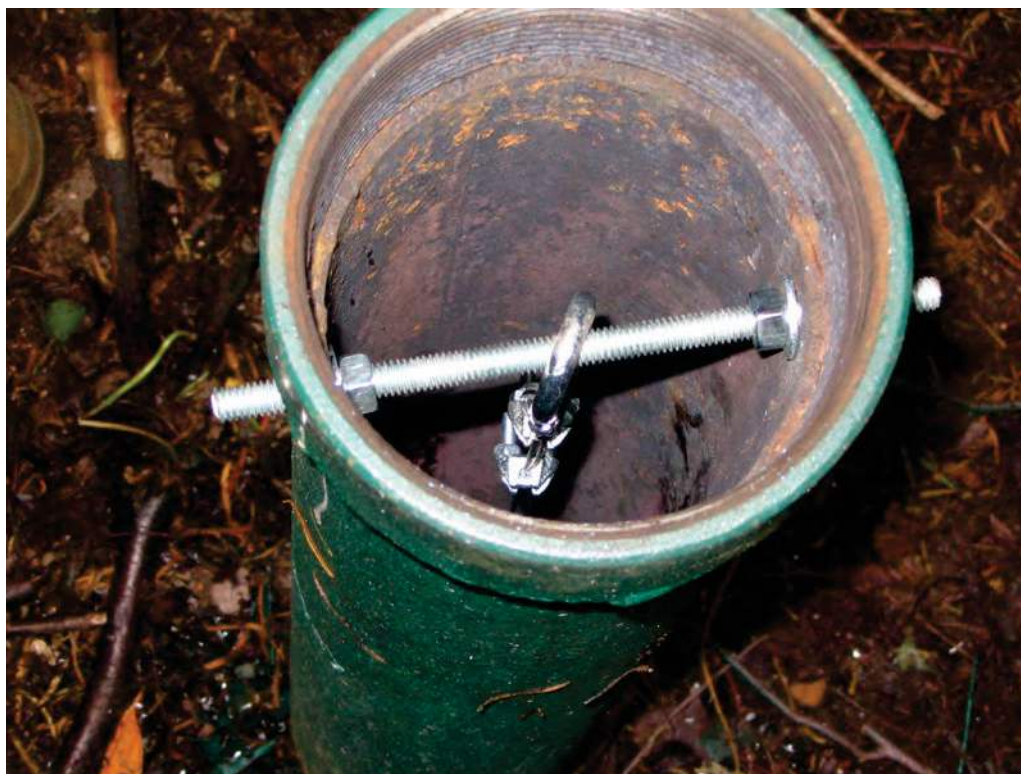
Figure 21. Tamper-resistant attachment of a weighted passive sampler suspension line to an interior bolt. Photograph by Thomas E. Imbrigiotta, U.S. Geological Survey.
