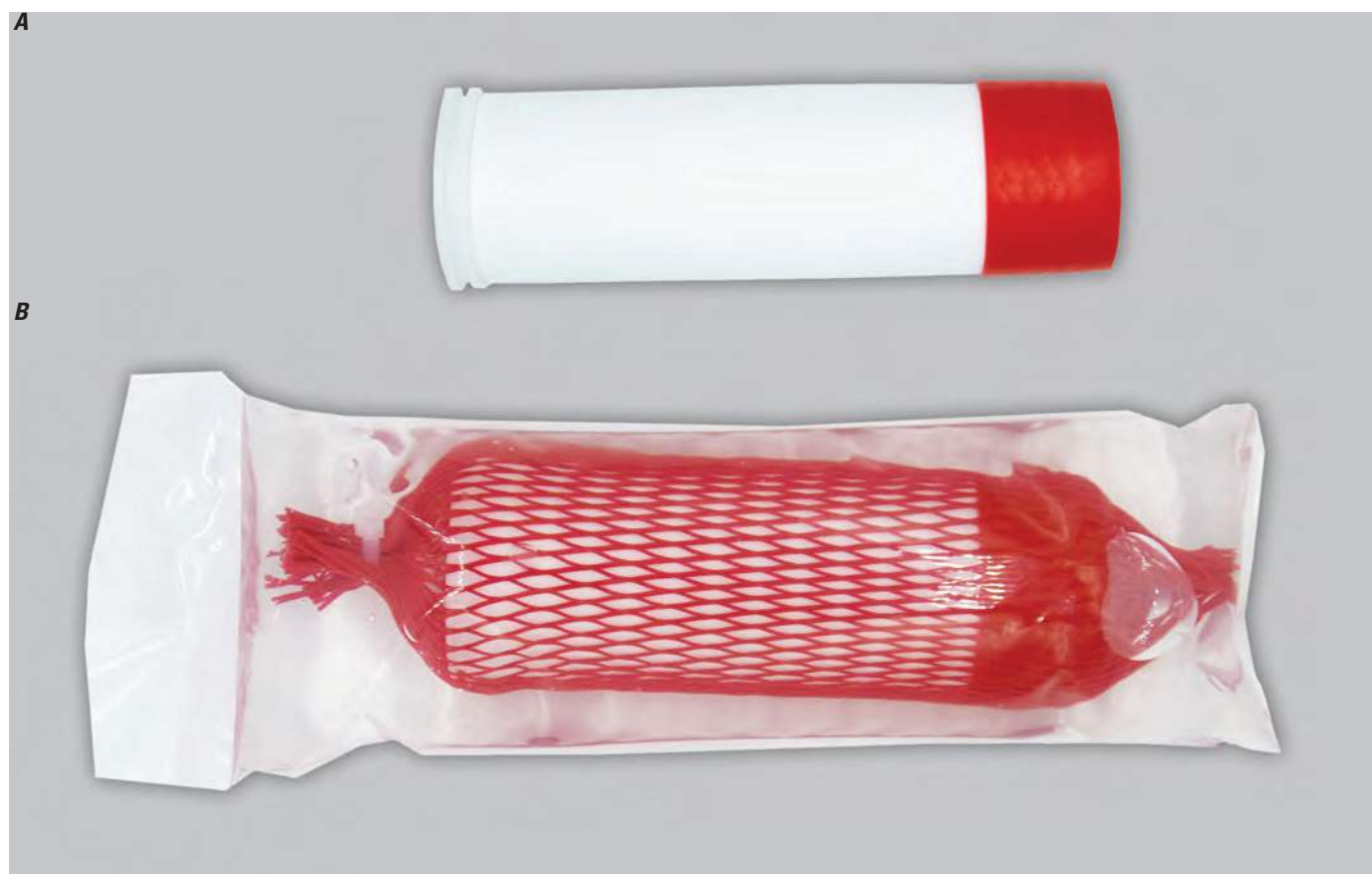
Figure 9. A rigid porous polyethylene sampler A , without the protective mesh, and B , with the protective mesh in a water-filled tube for shipment. Photographs by Leslie Venegas, ALS Global.
